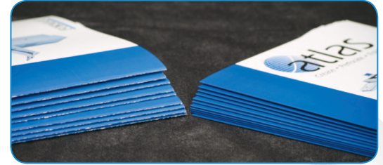
Uncreased folded digital prints (left) are cracked and give the appearance of poor quality. Creased prints (right) have no cracking and look polished and professional.
